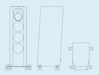
Frequency range / 24-100000 Hz +-2dB Power rating / 300 W Sensitivity / 87 dB / 1 m / 2.83V Impedance / 6 ohm (3.4 Ohm min) Type / 3-way bass reflex Drive units / 3x7" aluminium sandwich , 1x5" ceramic, 1x0.75" diamond Crossover frequency / first order: 370 & 4000 Hz Terminals / WBT Internal wiring / Jorma Design Cabinet / 25-40 mm:s fibre laminate cabinet Stands / Polished stainless steel with Marten pucks and cones Dimensions (WxHxD) / 28 cm x 107 cm x 38 cm (11" x 42.1" x 15")
